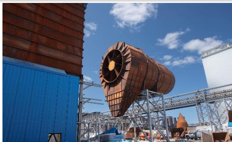
Axial Cyclone installation on Baghouse
